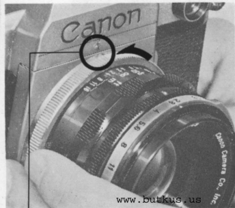
Coincide the red dots and remove
