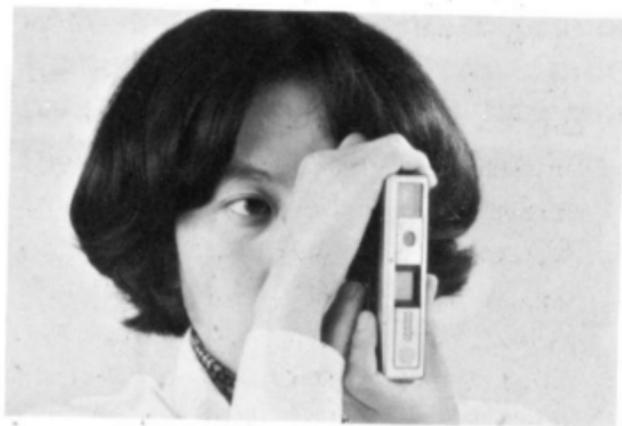
5. Depress the shutter release slightly. If the red light centered at the right side of the bright frame does not come on, hold the camera steady and continue to push the release all the way down to make the exposure.
