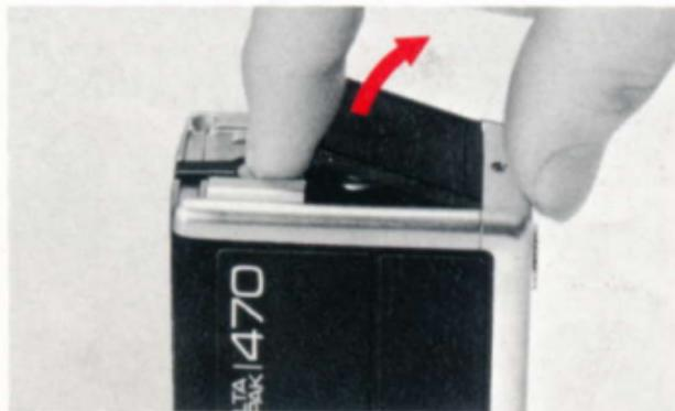
and minus (—) ends positioned as indicated inside the chamber, then close and latch the cover.
